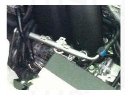
6.m. Connect the MAP and IAT connectors to the sensors, run and clip loom as per image below.
