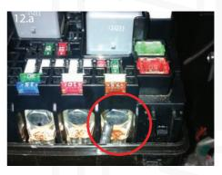
12.b. Feed the red positive wire (intercooler pump loom) up from LH opening where the side cover has been removed and install to the positive terminal shown in previous image and reinstall upper panel. Route the piggyback control wire inside the fuse box and out the inside of the side panel opening.
