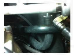
Connect the PCV vacuum line to the port on the engine block as shown (under the rear RH of the supercharger). Use the worm drive clamp supplied and secure (access to clamp is in east west plane and tightened by using a long screw driver or a ¼ drive socket with long extension from right side of vehicle).
