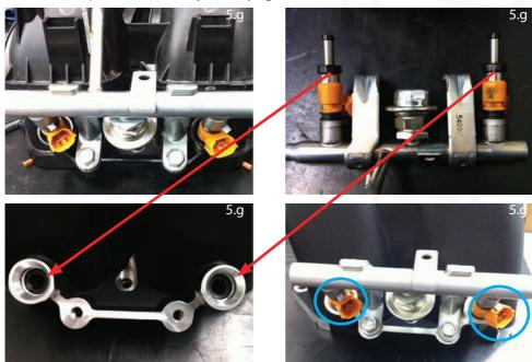
5.h. Transfer the MAP sensor from the original manifold into the supercharger manifold & secure using M5 screw provided.
