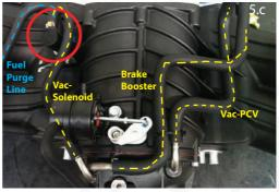
Note: For vehicles fitted with a seperate vacuum pump for the brake booster, fit the supplied cap and cobra clamp as shown and disregard hose marked in image 5.c.
