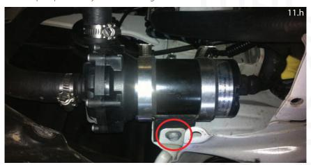
11.i. Connect the pump outlet A from the pump to the top fitting in the heat exchanger, connect the line from the engine bay (closest to the rail) to the lower fitting on heat exchanger, connect the remaining line from the engine bay to the pump inlet B using the #12 hose clamps. (For correct hose selection refer to CAD image at the beginning of the intercooler installation section on page 28).
