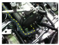
5.e. Move the grey loom and zip tie as shown. (remove connector from metal bracket to slip loom behind it).
