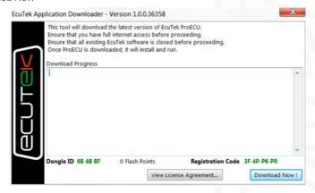
After the installation this bar should appear on your screen which is how the Ecutek software opens. Please note that if your interface cable and licence key are both plugged into your USB ports and you don't have 2 green bars or have any red in the bar you need to run the driver updated that pops up when first opening the app. (You will need to have internet access).
