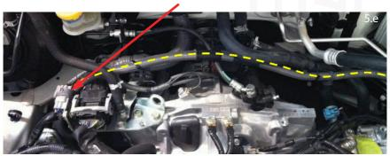
5.f. Install supplied throttle, MAP, MAF loom and route as shown (connect the supplied loom to the standard connectors and zip tie IAT loom to breather hose behind A/C compressor, throttle.
