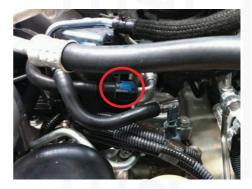
4.k. Remove the fuel rail support bolt from the LH fuel rail. 4.l. Remove the EVAP purge hose from the fuel rail fitting.
