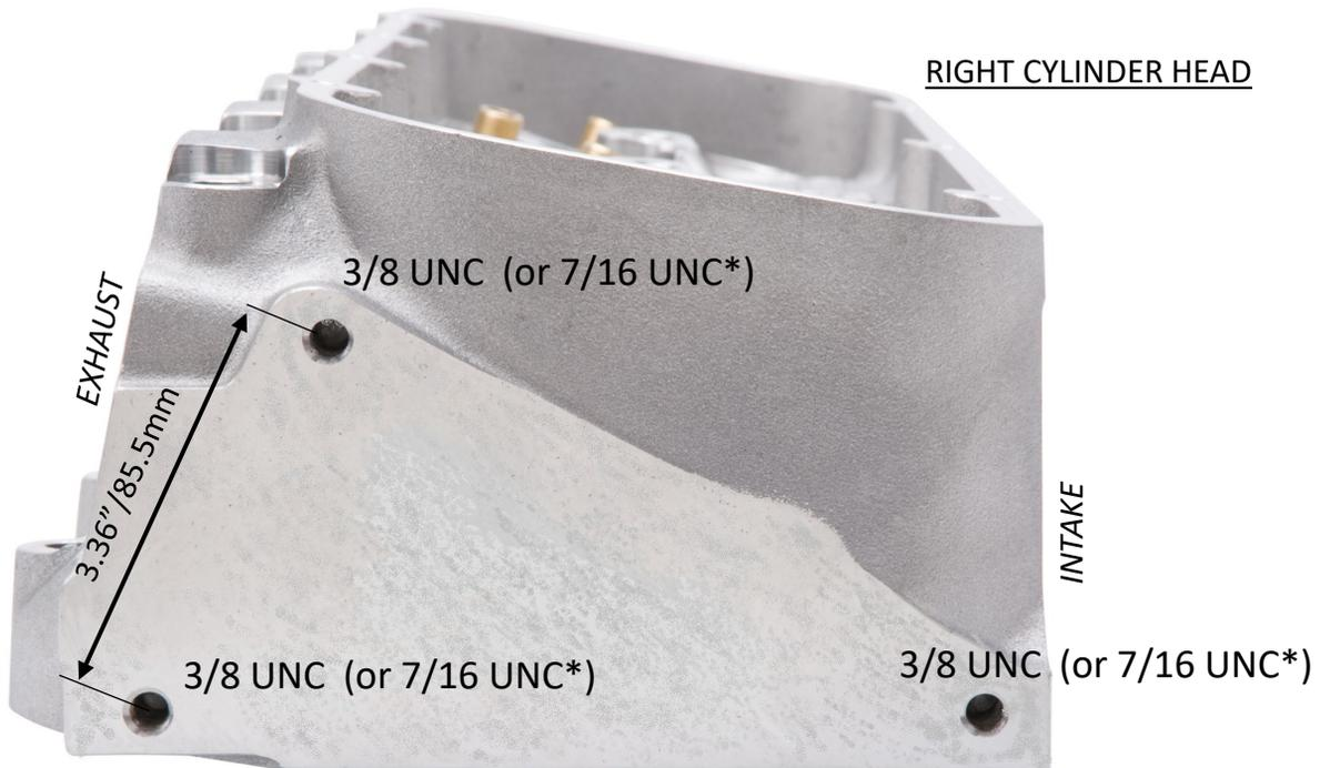
*\* Note: Drilling of optional A16415 Alternator Mounting kit maybe req'd to suit SHx7/16 UNC mounting bolts (not supplied) as thread specifications may vary across makes/models of cylinder heads.*
