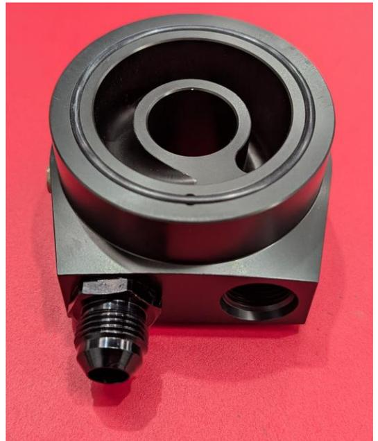
3. Apply oil to large o'ring on sandwich plate. Install the sandwich plate o'ring down where the oil filter was removed from. Thread female end of the sandwich plate fitting through sandwich plate into the male thread on the engine. Ensure sandwich plate ports face towards the left edge of the air box. Tighten sandwich plate fitting to 30 Nm torque.
