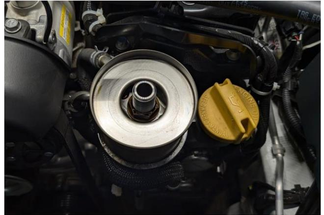
2. Assemble the dash 8 ORB to dash 8 fitting to the sandwich plate as shown. Apply lubrication to the o'ring and ensure fitting is fully seated.
