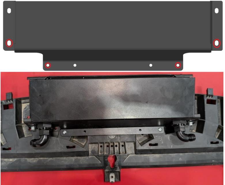
13. Remove left hand side infill panel and trim it as per image to allow oil lines to pass through. Attach pinch weld to the exposed edge.
