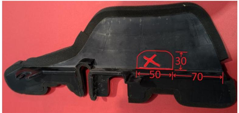
14. Drill air exit holes in lower under tray using a 60mm hole saw as per image. Ensure that the middle hole of the top row is centred on the undertray.
