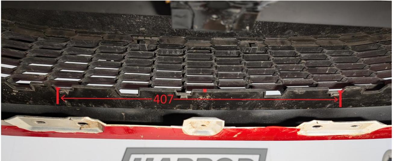
7. Trim the undergrille support piece as per the image below, ensuring the cut is centred.
