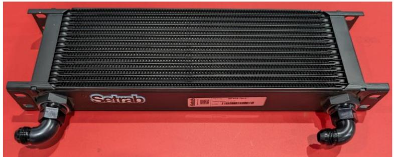
11. Connect short hose to left hand side of the oil cooler and long hose to right hand side of the cooler as per image.
