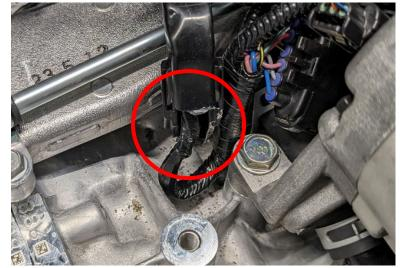
j) Install supplied throttle, MAP, MAF loom and route as shown (connect the supplied loom to the standard connectors and zip tie IAT loom to breather hose behind A/C compressor).
