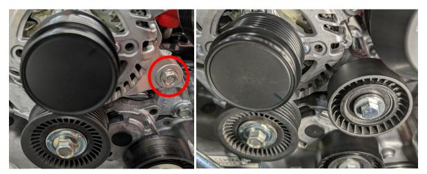
b) Using a 14mm socket and breaker bar on the belt tensioner install the supplied belt in the route as shown.
