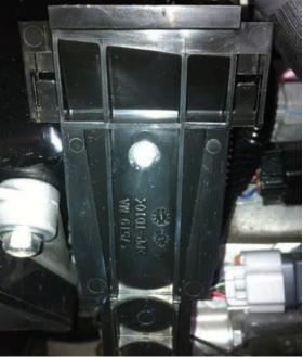
d) Remove the fuse shown. Install the fuse tap into the 15 amp EFI(IGN) fuse socket and route the wiring as shown and reinstall the fuse box cover.
