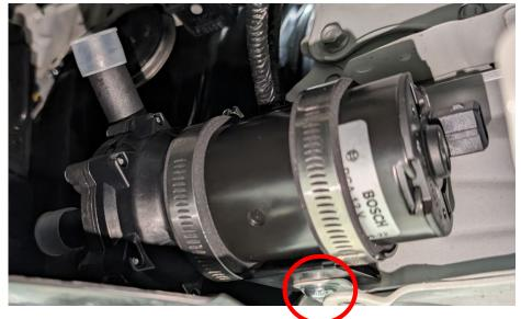
n) Connect the pump outlet A from the pump to the top fitting in the heat exchanger, connect the line from the engine bay (closest to the rail) to the lower fitting on heat exchanger, connect the remaining line from the engine bay to the pump inlet B using the 18-32mm hose clamps.
