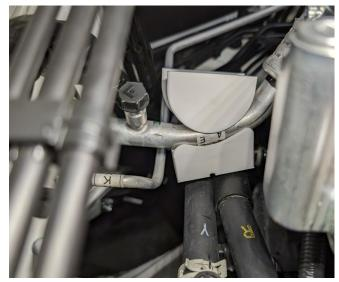
d) Using a G clamp or similar, clamp the tool bending the line to the correct angle.
