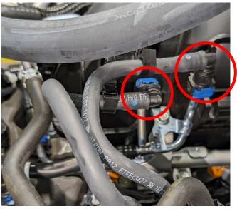
k) Disconnect the fuel crossover pipe from both fuel rails.
