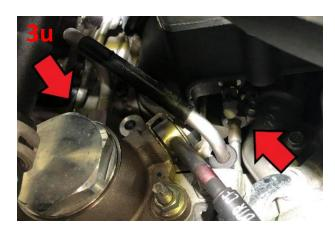
**3.v)** Replace the tensioner pulley with the supplied pulley. Re-use the OE bolt, which is a left-hand thread.
