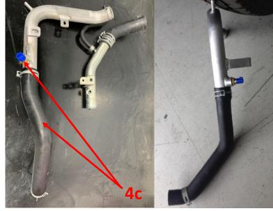
**4.d)** Fit the smaller end of the supplied reducer hose to the thermostat, re-use two OE spring-band clamps.
