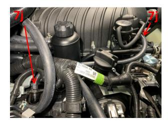
**7.k)** Re-Install the Engine coolant Reservoir, making the original hose connections.
