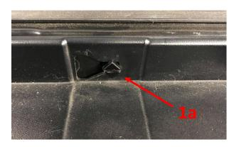
**1.b)** Next release the lower tabs by reaching through the opening through the front bumper and down both sides of the grille. Tab locations noted in image.
