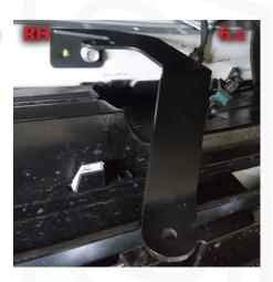
Note - MY18 cars and onwards mount the LH bracket on top of the radar mount.
