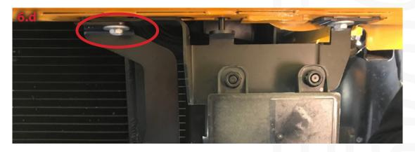
7. Insert the 2 U nuts into the lower front rails as per images 7.a and 7.b below. Mount the rear oil cooler mounting brackets as per image below but leave them loose. Note 'S' bend is to point forward - see image 8.a.
