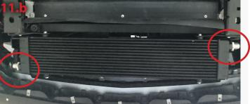
12. Route and connect the hoses onto the AN10 fittings as per image below, and cable tie off the hoses to the radiator and radiator hose.
